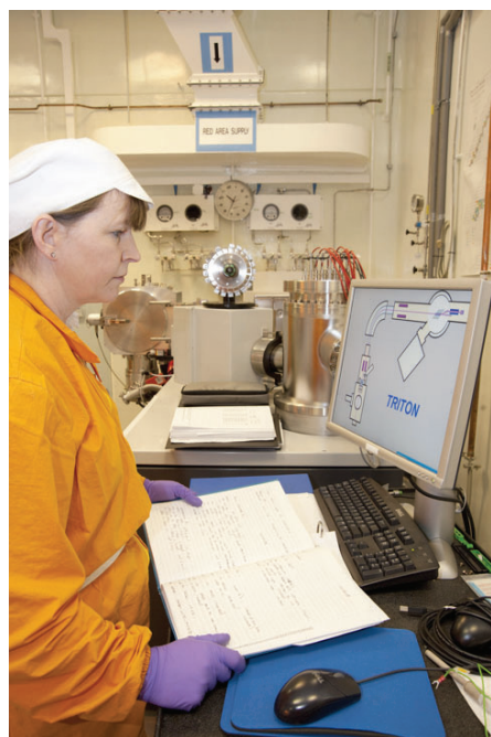
Fig. 4. The TIMS can quantify plutonium and uranium in comparable precisions while using smaller analytical samples.
