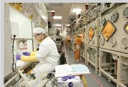
Fig. 1. This photo shows a typical actinide analysis facility, which consists of suites of gloveboxes and fume hoods.
