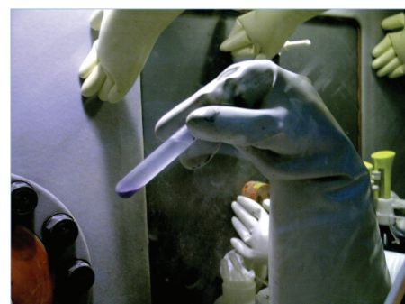
Fig. 6. This test tube holds Pu(III) oxalate precipitate.
