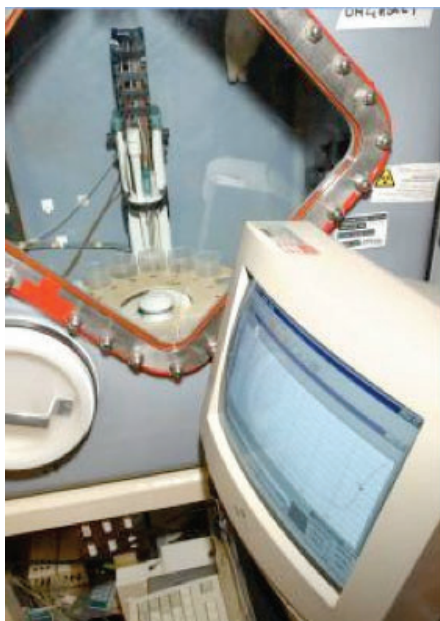
Fig. 3. This glovebox-contained autotitrator system is used to perform plutonium assay measurements.
